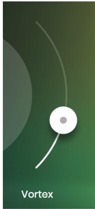
The Vortex slider creates the impression of sending the beat into a ... well ... vortex, whirling it around as you move the slider upwards. Use it to create mind-blowing risers and drops. From a technical perspective, Vortex combines an LFO-modulated notch filter sweep with compression.
