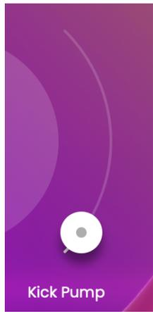
The Kick Pump control sends the Kick drum into a sidechain compressor, creating that typical super-compressed pump where the rest of the signal bows to the Kick Drum.
